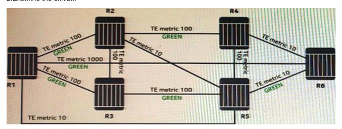
An LSP is being configured to start at R1and end at R6 using local CSPF. The LSP has the following constraints. Include admin-group GREEN, use the TE metric and hop-limit 3.
