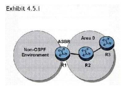
In the topology shown, router R1 is an ASBR configured to export external routes to OSPF. How many type 4 LSAs will be present in the network?
