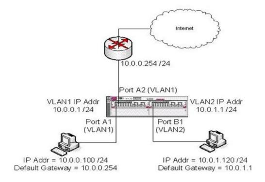
You need to limit the amount of broadcast traffic in this customer's network. In order to do so, you add a second VLAN, VLAN2 (10.0.1.0/24). Now, clients on VLAN2 cannot reach the Internet and cannot ping clients on VLAN1. They can successfully ping the default gateway (10.0.1.1). What should you do first to determine the cause of the problem?
