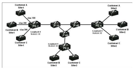
A provider of MPLS services offers multiple types of MPLS-based VPNs to its customers. Provider Edge router PE-1 directly connects to the following three customers:
