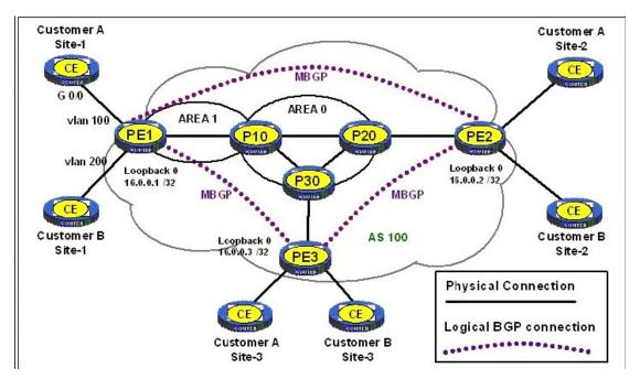
A provider of MPLS services configures MPLS Layer-3 VPN services for two customers. Each customer has three branch offices that will be interconnected by MPLS Layer-3 VPNs. The address blocks chosen by the customers for each site are shown in the following chart:
