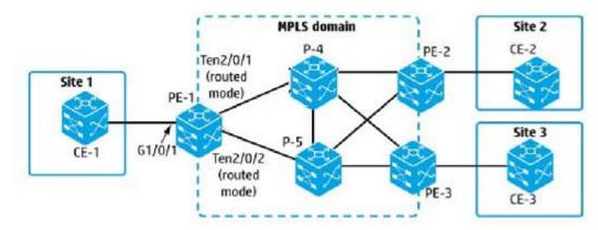
An administrator is setting up an MPLS Layer 2 VPN between customer Sites 1 and 2 and is defining the pseudo wire (PW) ID for this purpose. How should the PW IDs and router values be configured?
