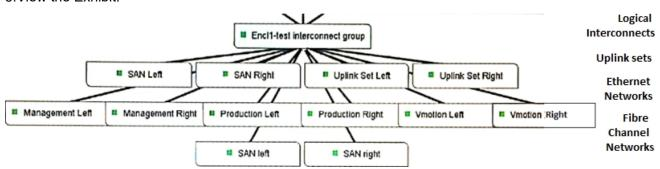
Refer to the exhibit. A customer has an HPE c7000 enclosure managed by HPE OneView with HP BL460c Gen9 servers in a vSphere cluster. The customer has multiple vLANs trunked from the top of rack (TOR) switches to the Virtual Connect modules in the enclosure. Due to network Access Control List (ACL) requirement and guidelines from the networking department, all network traffic should be forced to an upstream switch using the Virtual Connect "Private Network" feature.
