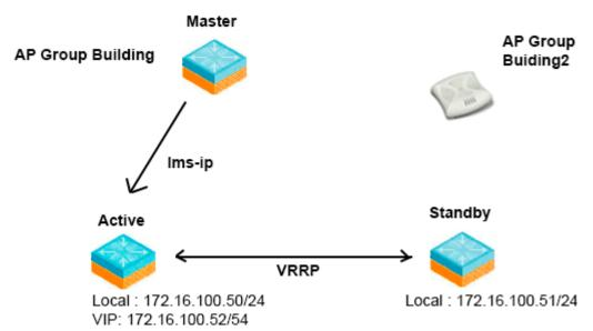
A network is configured with one master controller, one active local controller, and one standby local controller that use VRRP redundancy. All controllers are in the same center. The customer wants to configure AP termination redundancy in the event of controller failure and have the fastest recovery. How can the network administrator configure the controller for LMS redundancy to meet the customer's requirements?
