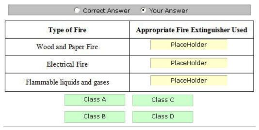
Explanation: Class A fire extinguisher is used for wood and paper fire. Class B fire extinguisher is used for flammable liquid and gases fire. Class C fire extinguisher is used for electrical fire. Class D fire extinguisher is used for combustible metals fire. Reference. "http://en.wikipedia.org/wiki/Fire\_extinguisher"
