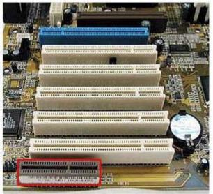
Explanation: Communication and Networking Riser (CNR) is a hardware device developed by Intel.It plugs into the motherboard and holds chips for the functioning of devices such as modems and audio devices.It supports V.90 analog modem, multi-channel audio, phone-line-based networking, and 10/100 Ethernet-based networking.CNR also minimizes electrical noise interference through the physical
