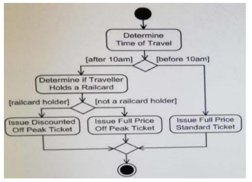
4. The following is an activity diagram of a trail company's rules determining ticket type.
